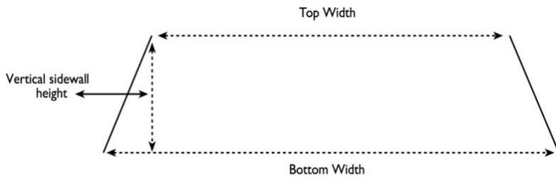
$$\frac{\text{Bottom Width} - \text{Top Width}}{\text{Vertical Sidewall Height}} < 0.50$$
